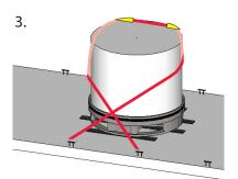
Continue to pass the webbing strap around the coil and bring to the 1st lashing point behind the coil winding axis.
