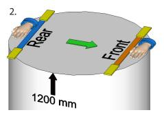
As the strap passes over the coil, position webbing sleeves at the edges.
