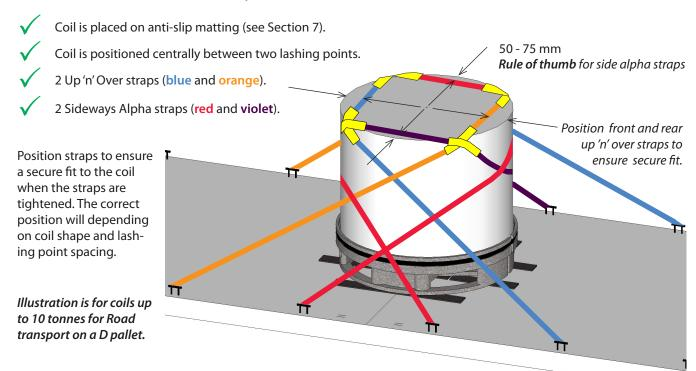
Note: Additional base straps are required for heavier coils, or coils moving on inter-modal rail routes (see Section 5).
