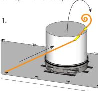
Attach a webbing strap to the 1st lashing point behind the coil. Bring the strap up to the front of the coil and pass over to the opposite side.
