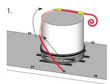
Attach a webbing strap to the 1st lashing point ahead of the coil winding axis. Bring the strap around the back of the coil and up to the top. Pass over the coil to the front.
