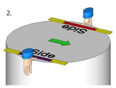
As the strap passes over the coil, position webbing sleeves at the edges.
