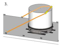
Continue to pass the webbing strap around the coil and bring the webbing strap to the lashing point opposite to the starting position.
