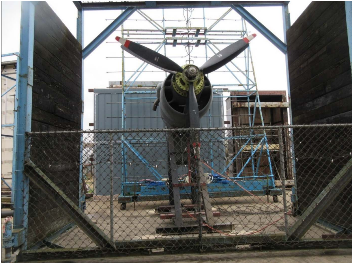
DYNAMIC WIND GENERATOR
